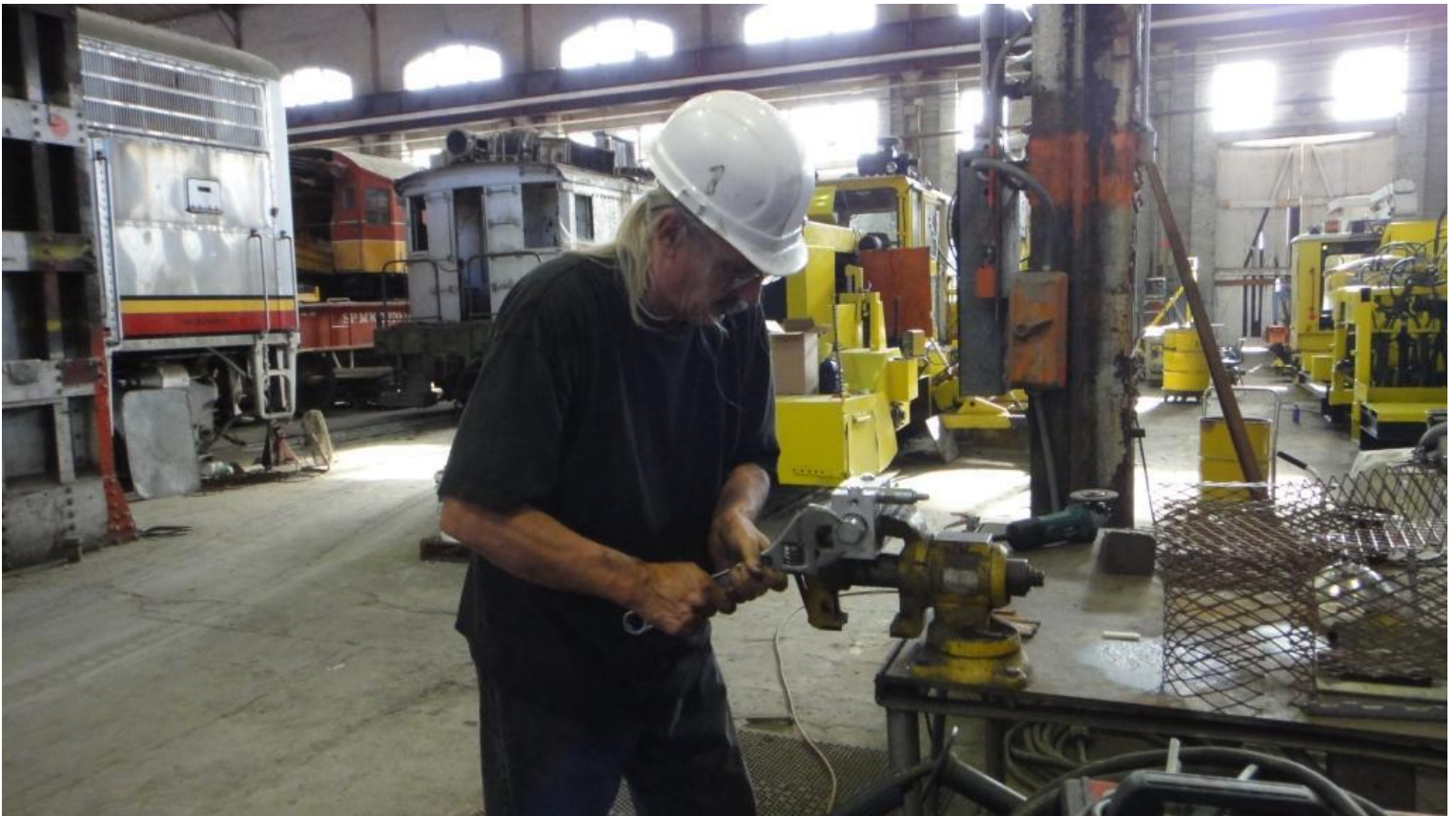
Fred makes adjustments to the multi-functional hydraulic valve on the tamper
