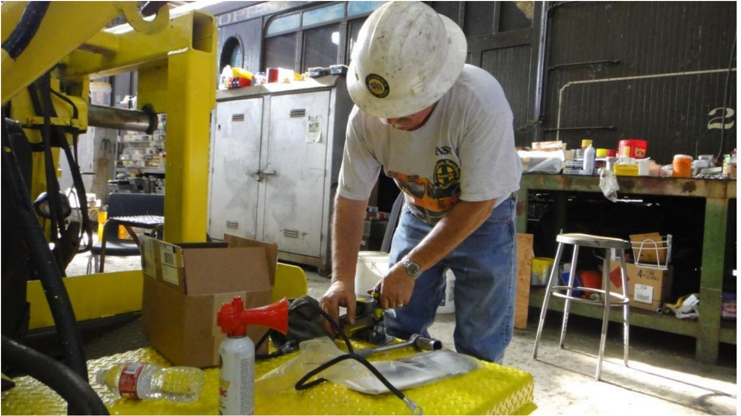
Mike H. adjusts the new solenoid for that engages the brakes on the Super B spiker
